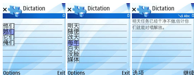
Figure 1 The input styles (from left to right: phrase input with 4 options, phrase input with 7 options and the sentence input)
